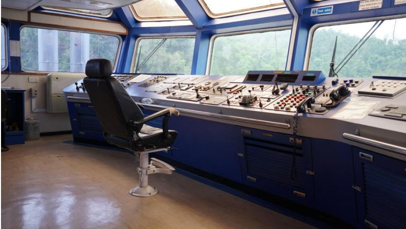
Aft Manoeuvring Console
